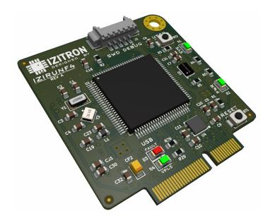
IZIRUNF4 is based on ARM Cortex-M4, designed for mid-power applications like motor control, display, CAN control, Ethernet, and more.
