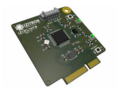
IZIRUNF0 is based on ARM Cortex-M0, designed for low power applications and IoT projects.
